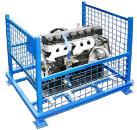
One tray as bottom layer loaded with a 6-cylinder engine in a pallet-cage
