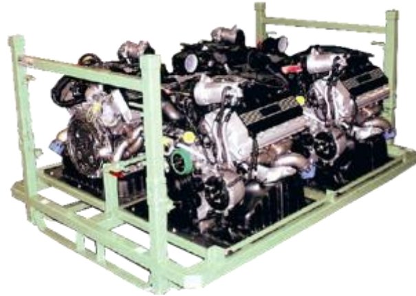
Two trays as bottom layer loaded with 8-cylinder engine in a steel load carrier
