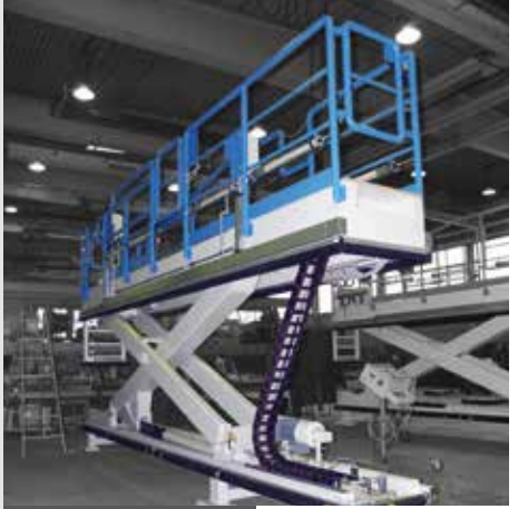
Work platform for painting aircrafts
