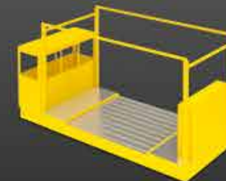
10 TRANSFER VEHICLE The transfer vehicle is used for transporting cargo horizontally on a single level. The individual loading units are moved on and off the racking by interconnecting the integrated roller conveyor with external roller decks. As well as transporting ULDs which can take up the entire surface of the roller deck, it is possible to transfer two containers simultaneously.
